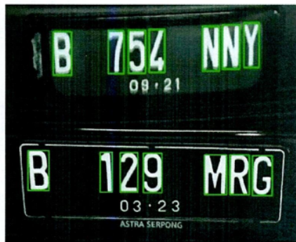
Fig. 4. Segmentation results of the detected license plate
