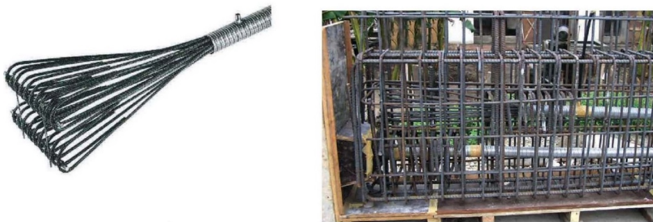
Gambar 6.5 Skematik sistem post-tensioned ( Dead Anchorage ).
