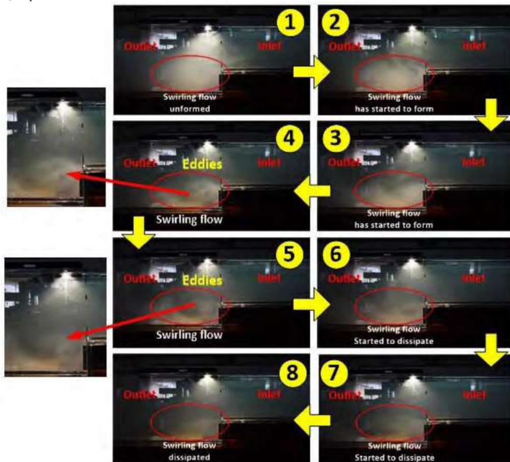
Figure 4. Captured flow at expansion zone
