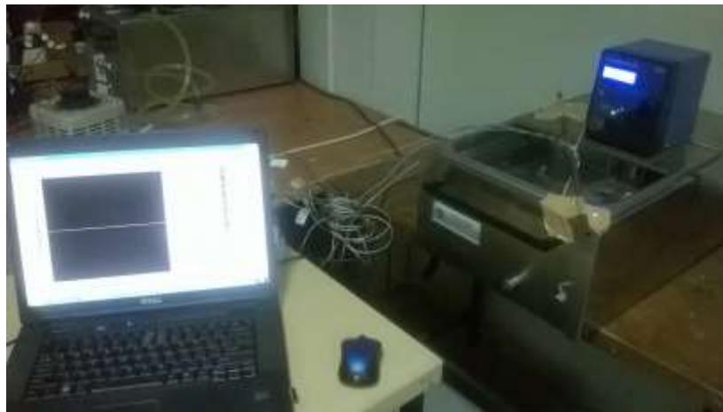
Gambar 3.10. Proses kalibrasi termokopel
