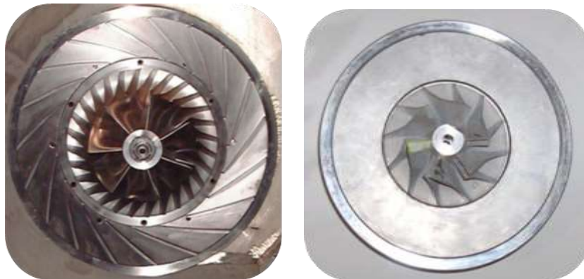
Gambar 3.3. (a) Vaned Diffuser [14] dan (b) Vaneless diffuser (Garrett TA31)
