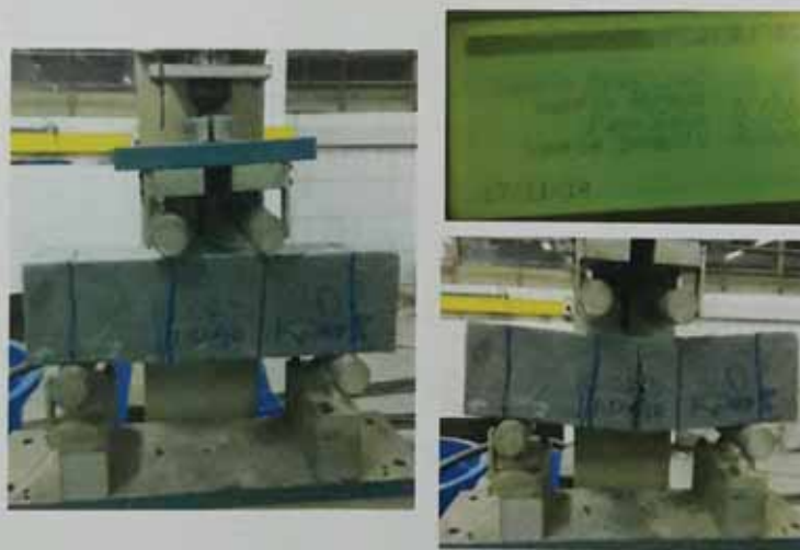
Fig. 6. Flexural strength test
