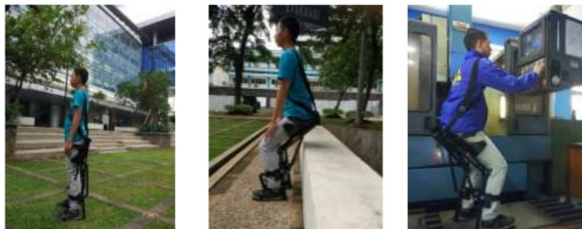
Figure 7. Field testing of the chairless chair [7], [8], [9]
