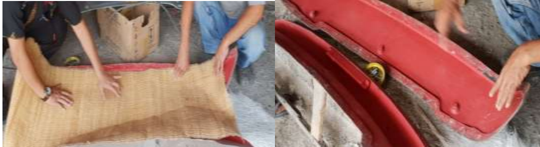
a. Preparation of rattan fibers and positive molds
